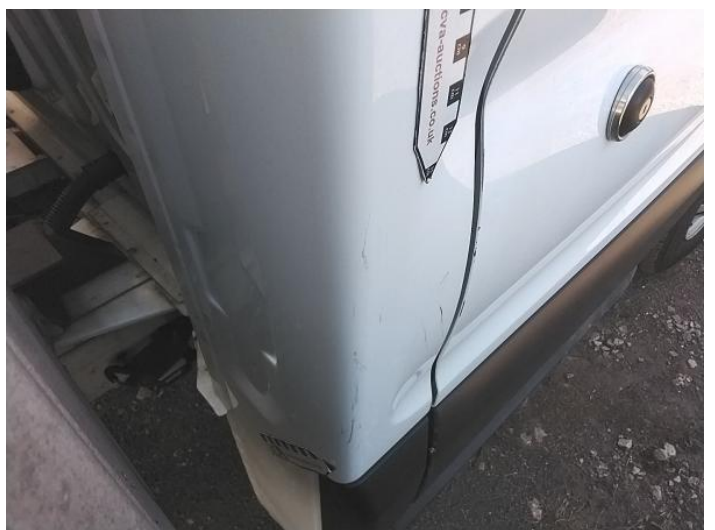
8: B Post os Scratched Over 25mm Thru Paint
