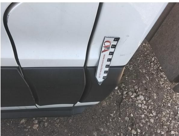
7: B Post ns Scratched Over 25mm Thru Paint
